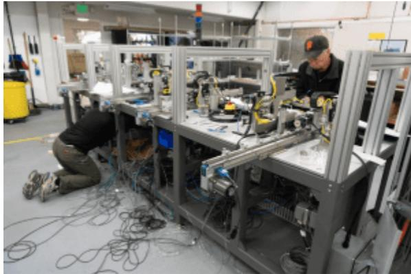
Automated assembly system for rapid medical diagnostic tests under construction at Kinematic
