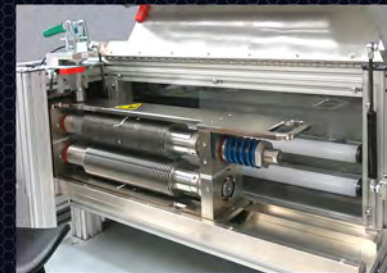
Slitting Module In Place
